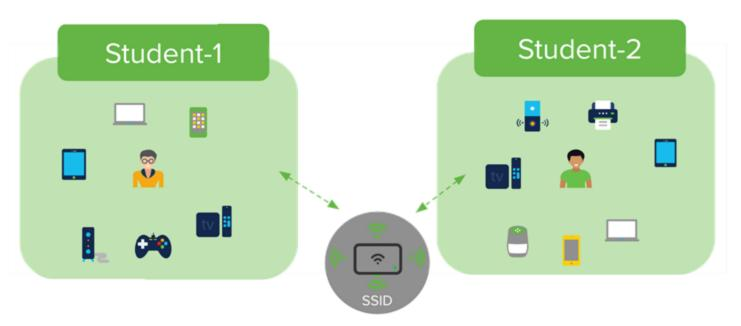
A WPN allows all user devices to authenticate to the SSID and communicate, creating a siloed personal network.
