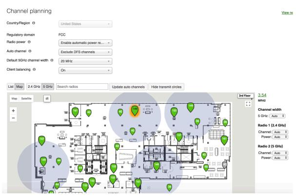
Figure 11. Fine-tuning a Meraki AP can include adjusting radio settings or configuring RX-SOP.
