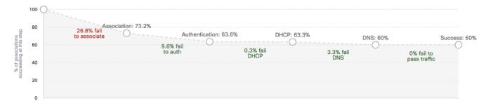
Figure 7. Meraki Wireless Health displays network-wide failures across each stage of client connectivity, allowing rapid root cause identification of poor network performance.
