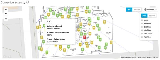
Figure 8. AP 5.10 is primarily experiencing authentication failures.
