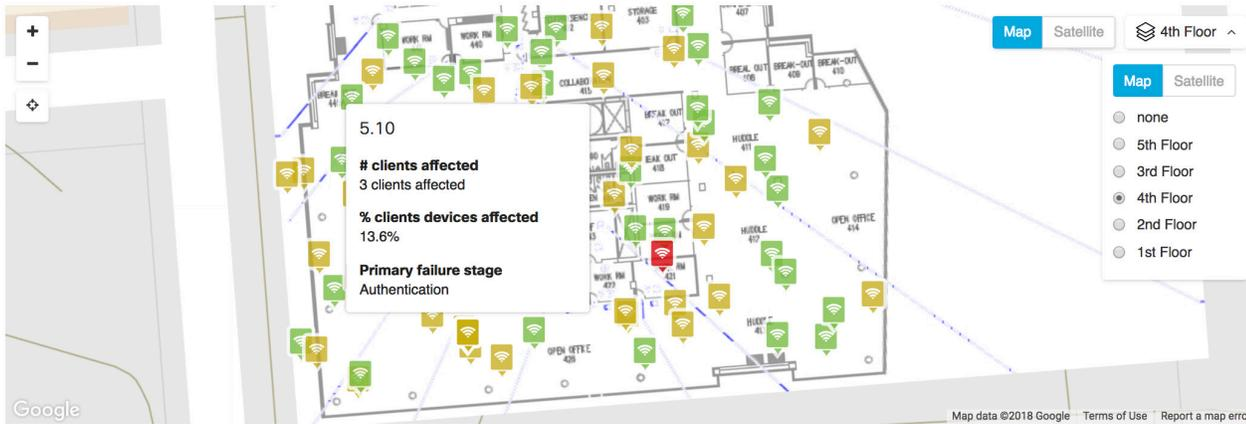
Figure 8. AP 5.10 is primarily experiencing authentication failures.
